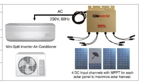
Product: CyboInverter - 4 Channel 1.2KW Off-Grid Solar Power Mini-Inverter CI-Mini-1000Rx Standalone Off-Grid Model for 230V, 60Hz IAC Units
