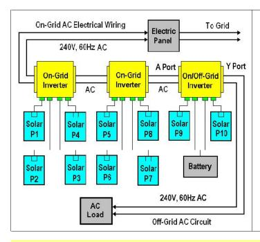
When the grid is on, the inverter works like a regular on-grid inverter that meets UL1741 and IEEE1547 standards including: over and under voltage shutdown; over and under frequency shutdown; and anti-islanding.
