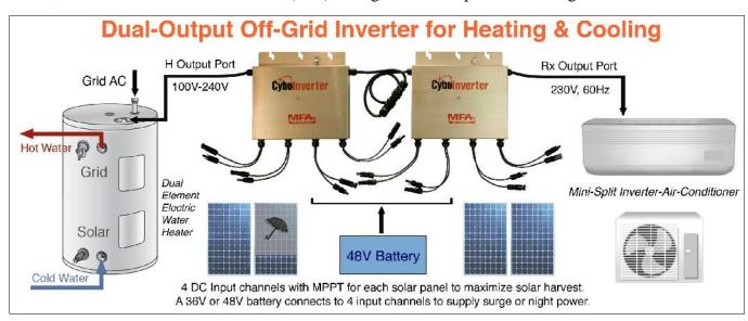
Product: Dual-Output Off-Grid CyboInverter Twin Pack for Microgrids CIM-1200H/R1x, H/R2x, H Port: 100V-240V, Rx Output Port: 230V, 60Hz
