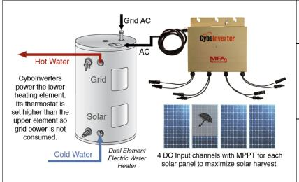
Solar Heating for Single Element Water Heaters, Air Heaters.
