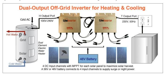
Product: Dual-Output Off-Grid CyboInverter Twin Pack for Microgrids Part No: CIM-1200H/T1, H/T2, H Port: 100V-240V, T Output Port: 230V, 50Hz
