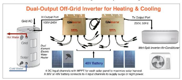
Product: Dual-Output Off-Grid CyboInverter Twin Pack for Microgrids CIM-1200H/T1x, H/T2x, H Port: 100V-240V, Tx Output Port: 230V, 50Hz
