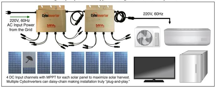
**Product: AC Assisted Off-Grid CyboInverter Twin Pack (8 Input Channels)**
