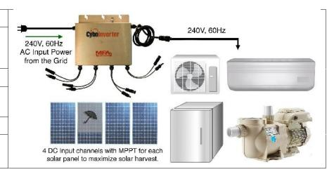
Product: CyboInverter - 4 Channel 1.2KW AC Assisted Off-Grid Solar Inverter CIM-1200Ya Standalone Off-Grid Model for 230V-240V, 60Hz AC Loads.
